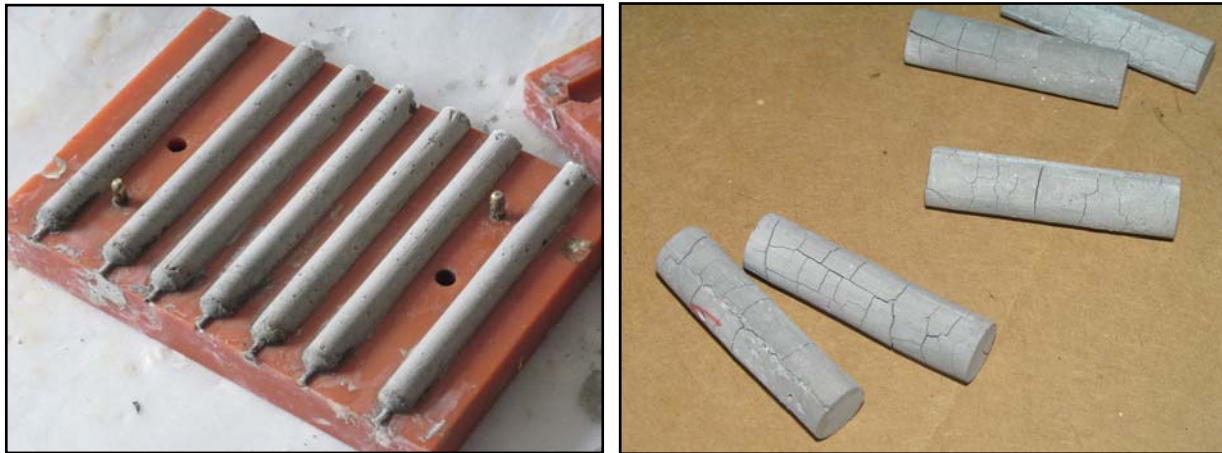
Fig. 1: The samples in the mould after 48 hours (left), after loading by temperature of 450 ° C with visible cracks (right).
