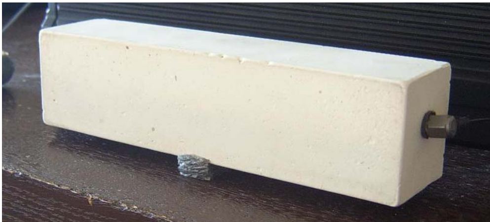
Fig. 1: Measurement of the natural frequency of longitudinal vibration.
