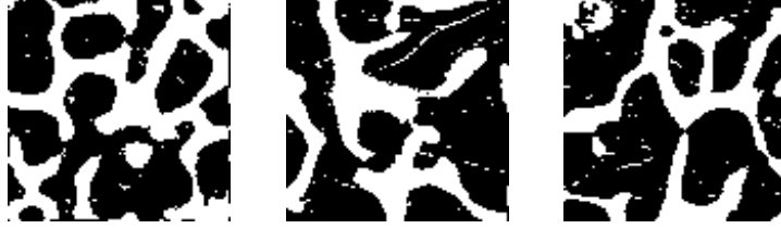
Fig. 1: Three cuts through trabecular bone microstructure obtained by micro Computed Tomography (Jiroušek et al., 2008), courtesy of O. Jiroušek, Institute of theoretical and applied mechanics.
