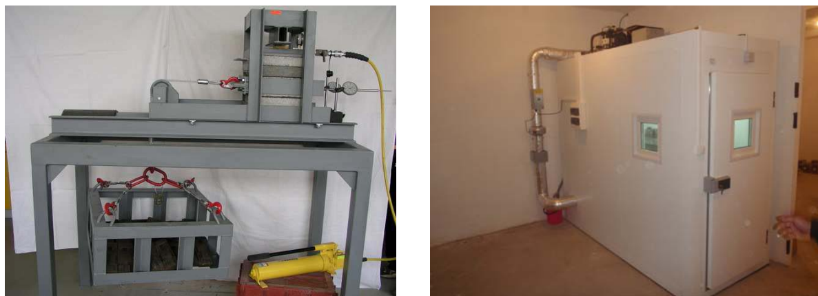
Fig. 2: Testing rheological shear characteristics in air conditioned room.
