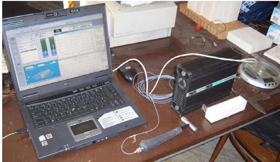
Fig. 2: Measurement line for the Impulse Excitation Method.
