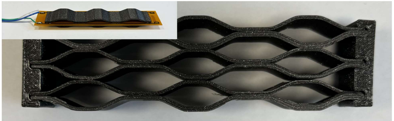
Fig. 4: Three base unit testing sample and a planar three-layer concept smart structure.
