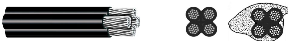
Fig. 1: Bundled overhead line – axonometric view, cross-section and ice-covered cross-section.
