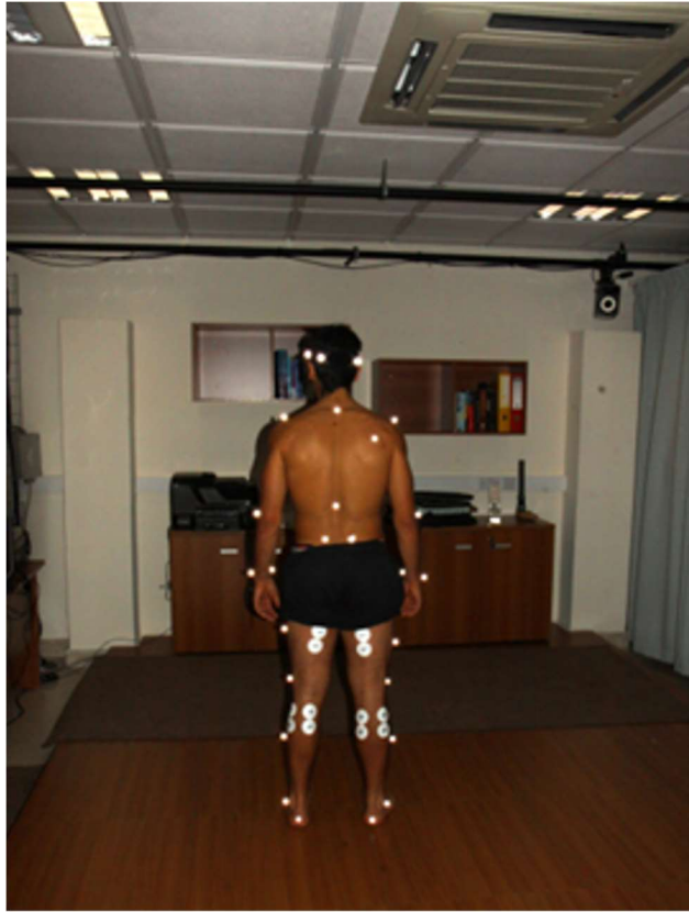
Fig. 10: Subject with markers and attached sEMG device.
