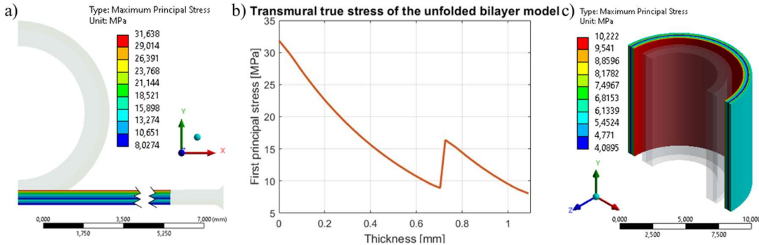
Fig. 3: a-b) Unfolded bilayer model, a) stress at the end of the simulated test, b) transmural true stress; 0 mm - inner edge of media, c) cylindrical model after inflation.
